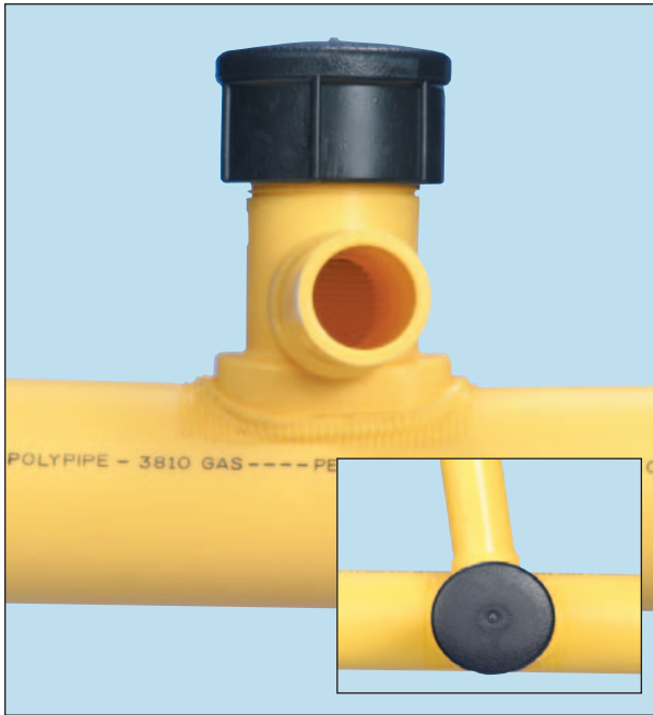
Fitting misaligned on pipe.
