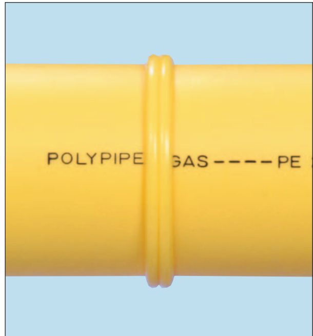
Melt bead too large due to excessive heating and/or over-pressurizing of joint.
