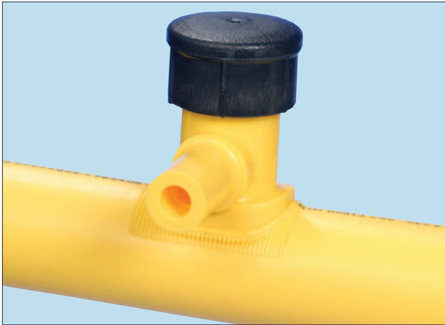
Proper alignment, melt and force.
