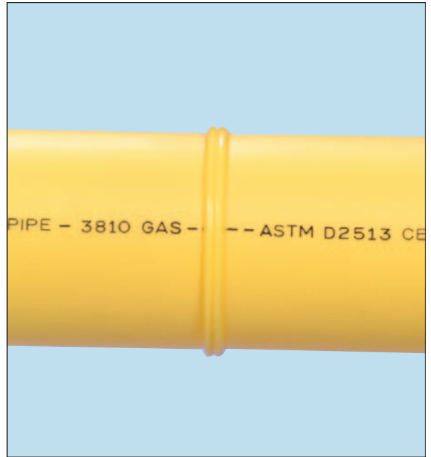
Proper alignment and double roll-back bead.
