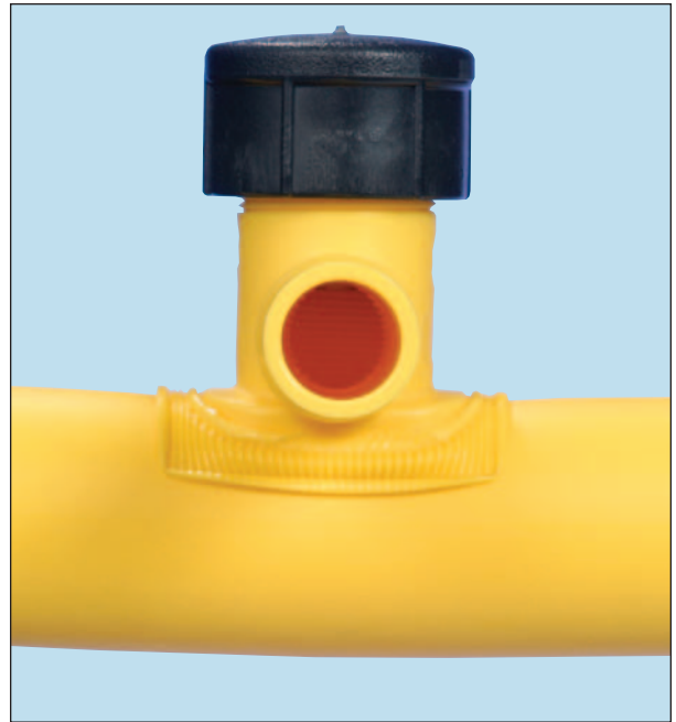
Excessive heating and/or over-pressurizing of joint.
