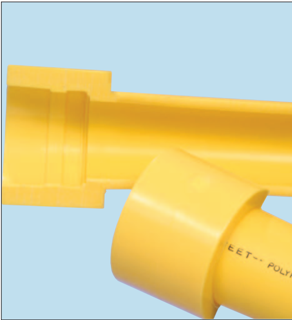
Short stab depth caused by failure to use a depth gauge.
