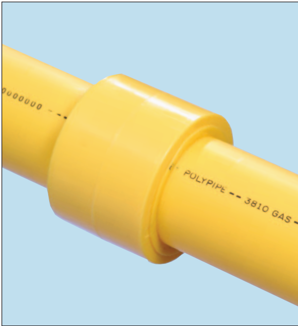
Proper alignment and stab depth. Melt bead flattened due to cold ring. No gaps or voids.
