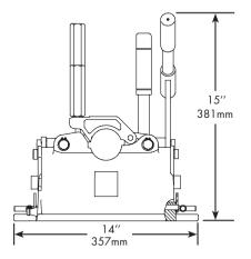
weight 23lbs (10.4kg) input power 800 Watts
