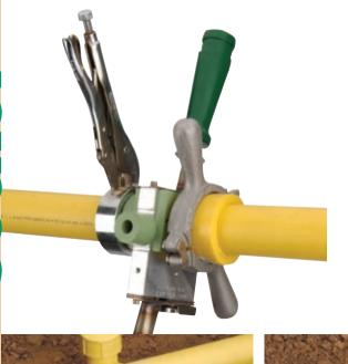
**McElroy Socket Tooling** allows socket fusion of 1/2" CTS – 4" IPS pipe. Select the heater, heater adapter, depth gauge/chamfer tool, and a cold ring tool for your application. For 2" and larger fittings, a socket fitting holder is required. Socket heater adapters are available for 1/2" CTS – 4" IPS.
