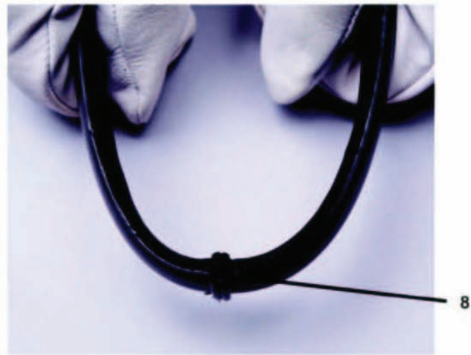
8. No gaps or voids when bent
