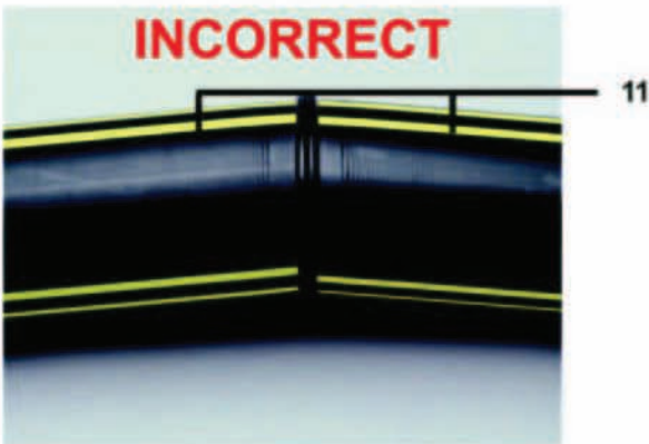
11. Pipe angled into fusion unit
