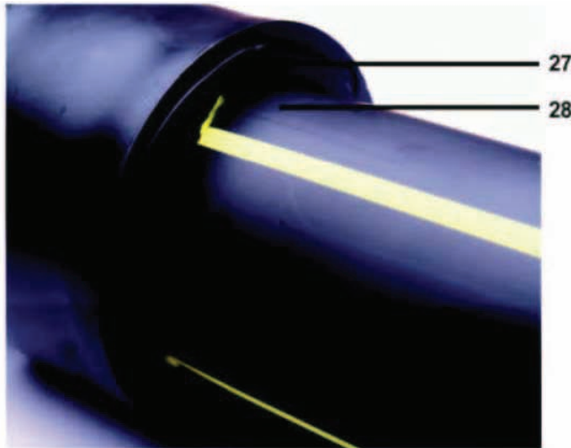
27. Melt bead flattened by cold ring 28. No gaps or voids
