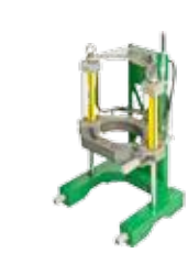
DYNAMIC 28 SIDEWALL Max. Fitting Base Diameter 9.63" (245mm)
