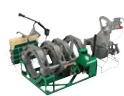
DYNAMIC 412 HP (HAND PUMP) 4" IPS - 12" DIPS (110mm - 340mm)
